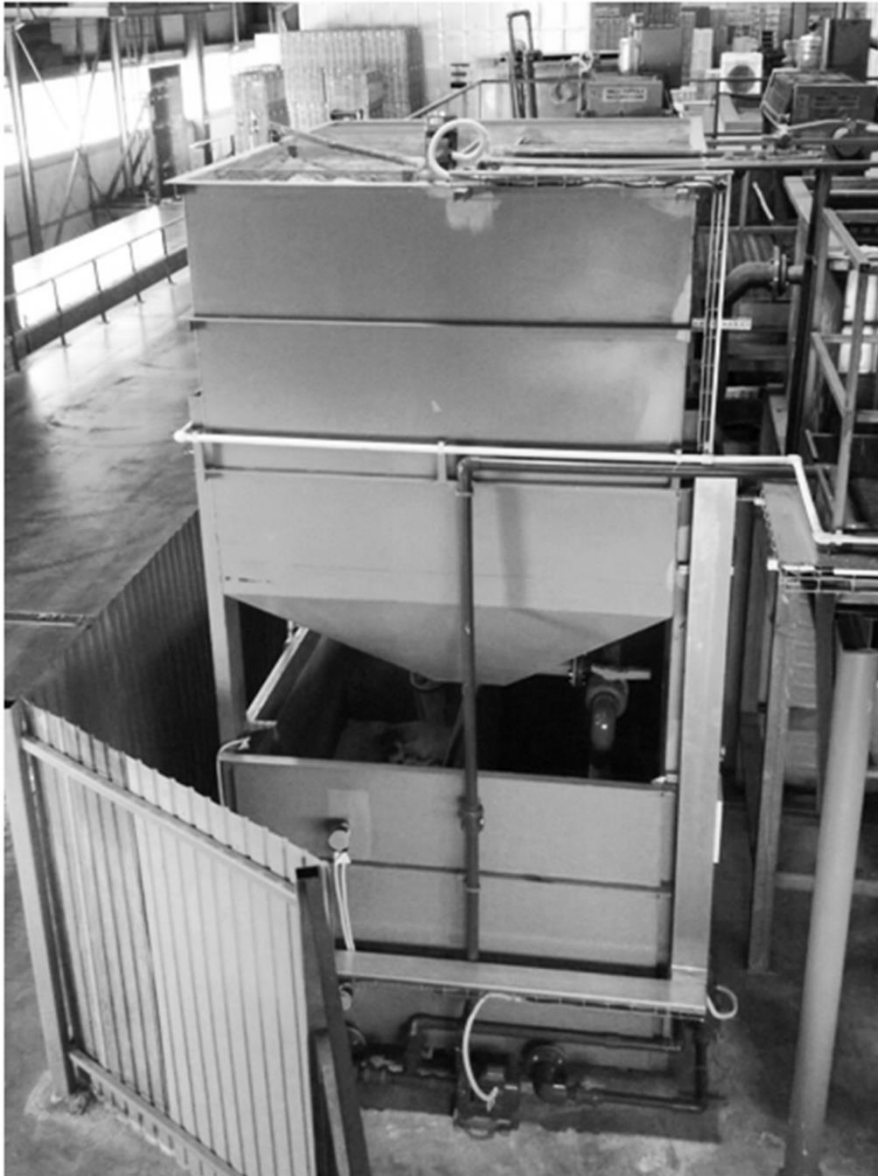
Fig. 2.13. Photo of an industrial sample of a flotation settling tank
