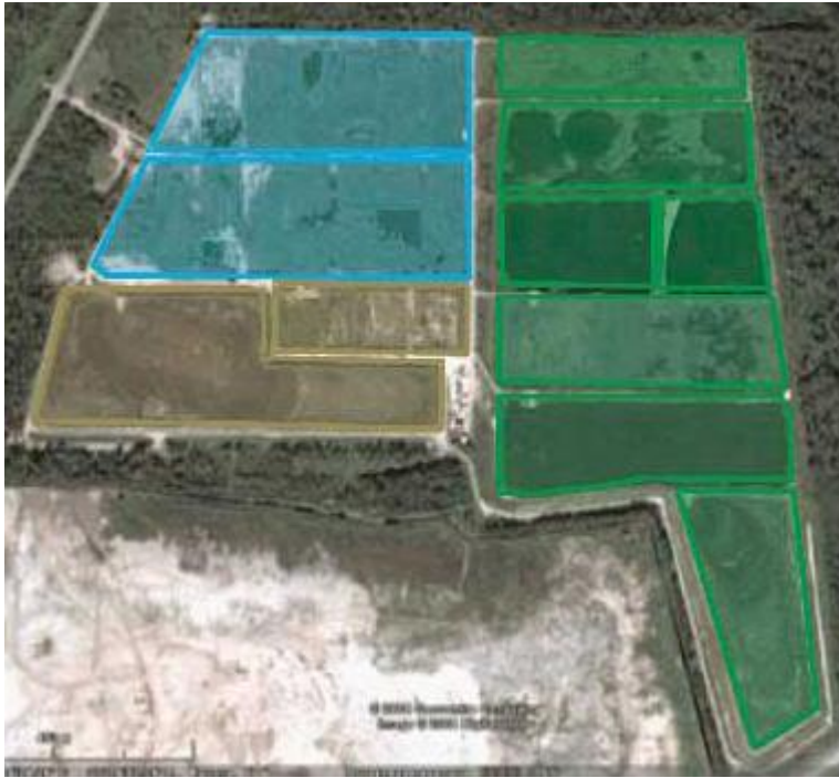
Fig. 10.3. The planned results of the application of the technology of geotubation of sediment - the territory for the storage of ash and technological waste (a reserve for 25 years is provided); - the released territory for the creation of a protective forest belt; -
